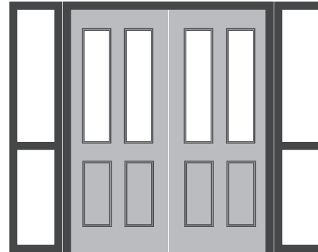
Double Doors with Glazed Sidelights and Midrails
